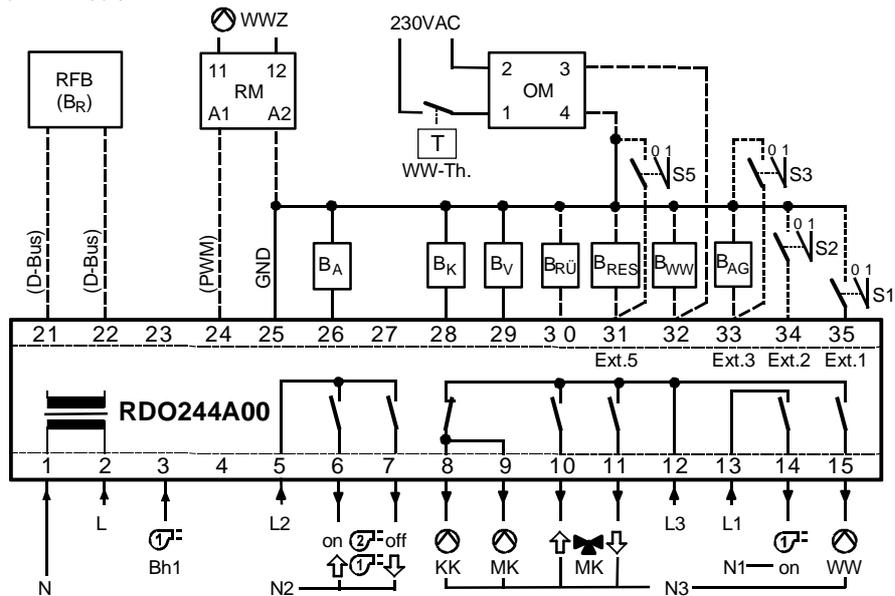
**The function of the inputs (switch functions) is configurable!**
